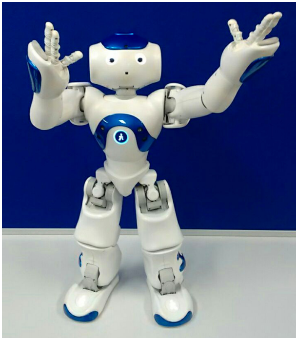
Figure 1: The Nao robot from Aldebaran. In this image, the robot performs a gesture titled ShowSky_1 that has been associated (with medium strength) to the actions: look up, praise, pray, preach and worship.
