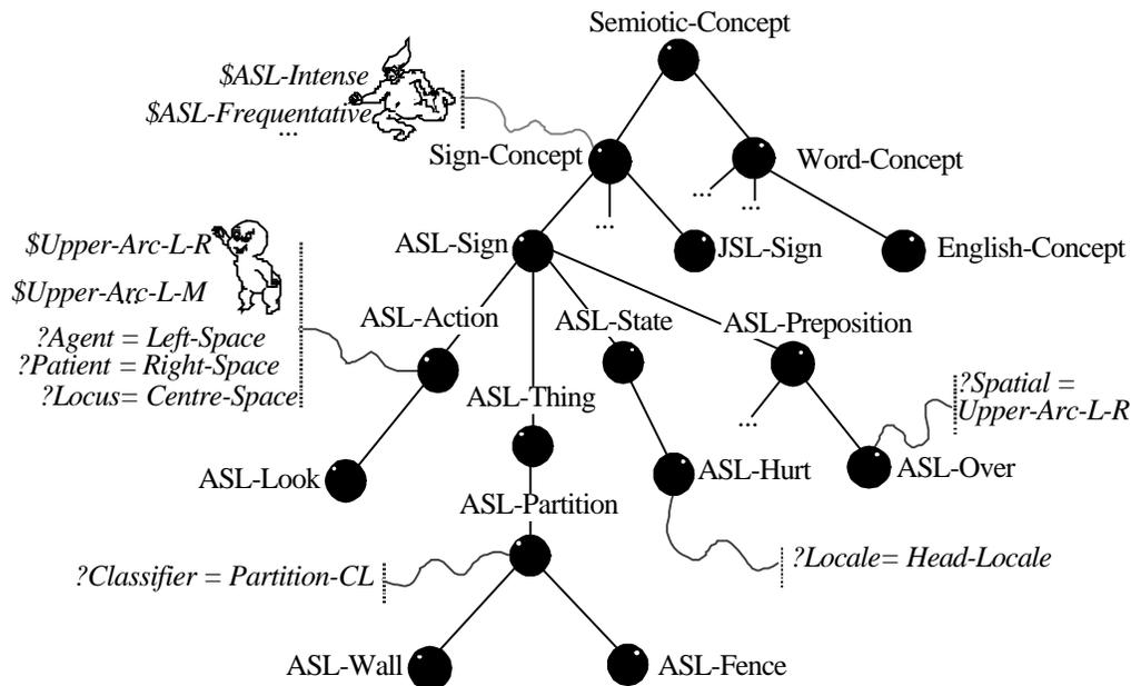
Figure 9: The ZARDOZ Concept Network and Object Hierarchy. Statements prefixed with “?” indicate local DCL variable assignments, while tokens prefixed “\$” indicate demon attachments for given message types.
